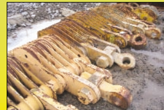
100 ton NYE blocks 6 sheave
